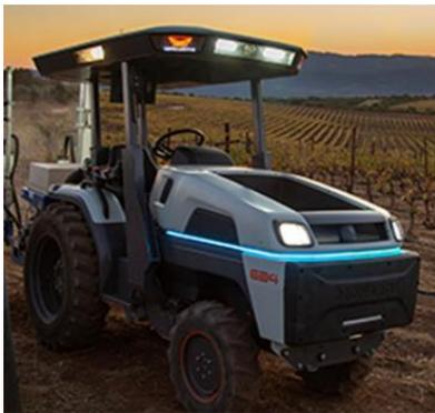
Being 100% electrical, the Monarch Tractor has zero tailpipe emissions -- unlike many of its predecessors. With extra storage, the e-tractor can act as a sort of ATV and work as an ad hoc power generator in the field.
