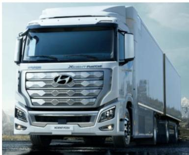
XCIENT trucks are powered by a 190 kW hydrogen fuel cell system with dual 95 kW fuel cell stacks. Seven large hydrogen tanks offer a combined storage capacity of around 32.09kg of hydrogen.
